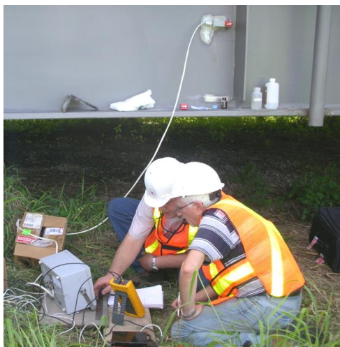
Fig.10. Process of measurement of residual stresses in a welded bridge
