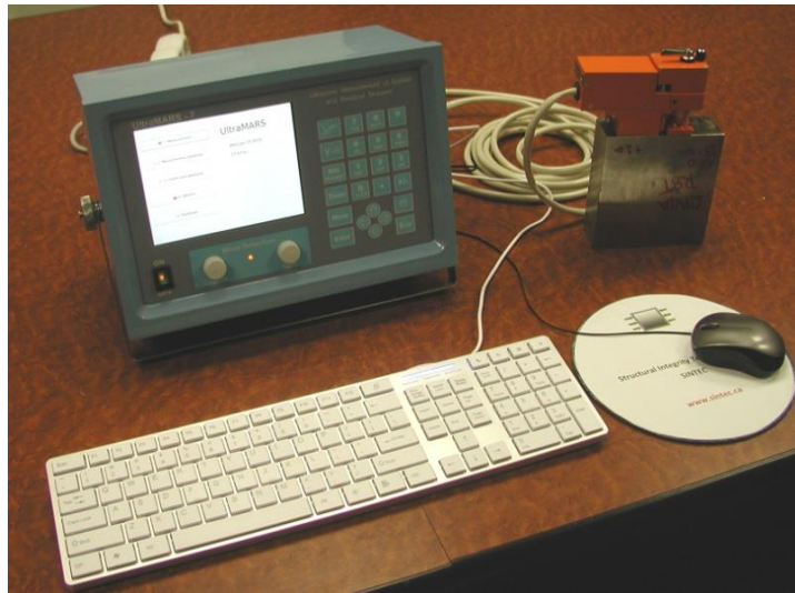
Fig. 4. Ultrasonic Computerized Complex for residual and applied stress measurement.
