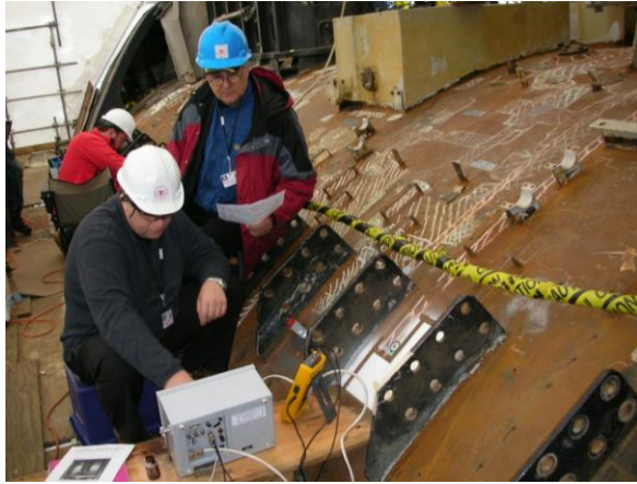
Fig. 12. Residual stress measurement in one of the welded elements of the pressure hull of a submarine
